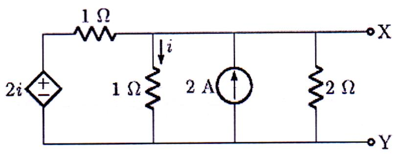
47. In the circuit shown, what value of  $RL$  maximizes the power delivered to  $RL$ ?
